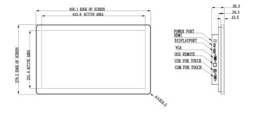
**Specifications** DG1850-0006-C810 Part number Enclosure color Black 409.8mm (H) x 230.4mm (V) / 16.13" x 9.07" Active area Diagonal 18.5 inch Aspect Ratio 16:9 Resolution 1366(H) ×768(V) 640x480 60Hz; 720x400 60Hz; 800x500, 60Hz; 800x600 60Hz; 1024x768 60Hz; Other Supported Resolutions 1280x80060Hz; 1280x1024 60Hz; 1366x768 60Hz, 60Hz RB; **Number of Colors** 16.7M LCD panel: 300 nits Brightness (typical) Response Time (typical) 8ms 178°(H); 178°(V) Viewing Angle 89°(H)
