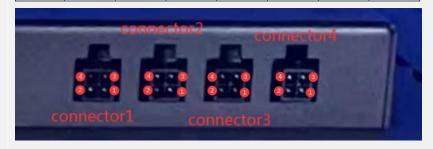
Note1:The pin of the connector 2 is connected to tail end of the first RGB light strip
